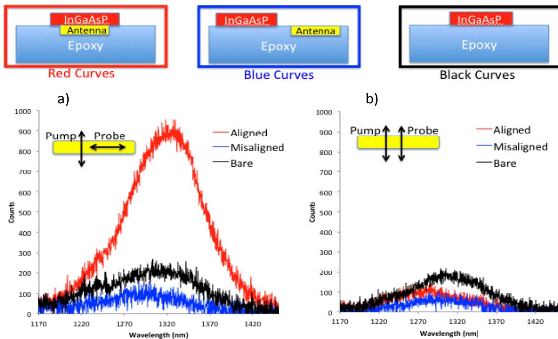
Fig 2. Spontaneous emission spectrum from aligned (red), misaligned (blue) and bare (black) devices. a) emission parallel to the long axis of the antenna, b) emission perpendicular to antenna
