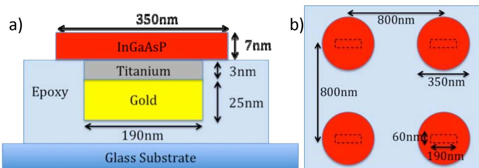
Fig 1. a) cross-sectional view of the fabricated structure, b) top-view
